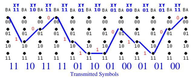
Upon reception, it is necessary to reconstruct the original bitstream essentially by retracing the above path from the symbols which are received. Error correction is possible because an errored symbol will cause a detectable deviation from the correct path. The remaining symbols may be then used to reconstruct the most likely correct path and consequently, the correct bitstream. This process is explored in the next section.
