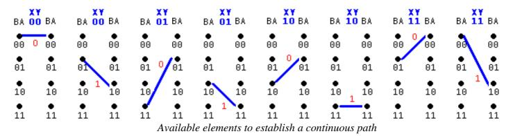
Proceeding by trial and error to find the "missing symbols" presupposes that the location of the bad symbols was known and greatly oversimplifies the decoding process. *Perhaps the symbols leading up to the "obvious" break in the path are themselves incorrect.* In general, **the exact location of any bad symbols cannot be known in advance**. In practice, a systematic approach to identifying the best path through the trellis can be employed to correct errors automatically as they occur.
