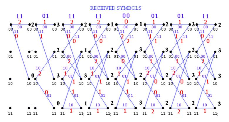
At the end of the table (far righthand side) there is one path which gives the lowest cumulative error (2). In fact, this path corresponds to the correct data. The above algorithm could be easily be carried through if the message were to continue from this point.
