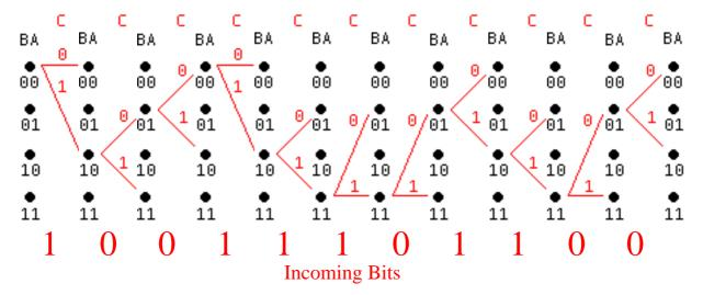
The exclusive-OR circuitry maps a two-bit symbol (XY) onto each of the above state transitions. The trellis diagram can now be redrawn to show the symbols associated with the above states.
