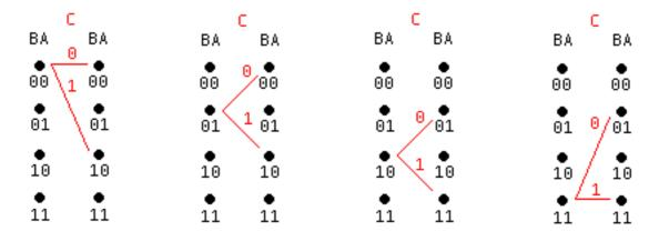
The effect of the exclusive-OR may now be included. Each three-bit condition (CBA) is associated with a unique two bit "symbol" (XY), the behavior of the circuit in time can be summarized in the table below. As as each new bit arrives one of two possible two bit "symbols" is generated as a function of the bit (C) and the shift register state (BA).
