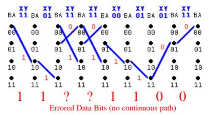
It is necessary to reconstruct a continuous path from the above information. The "best fit" path will be the one which best matches the above data, deviating only as required to establish continuity. The available resources to establish this path are the four possible symbols and the corresponding eight possible state transitions:
